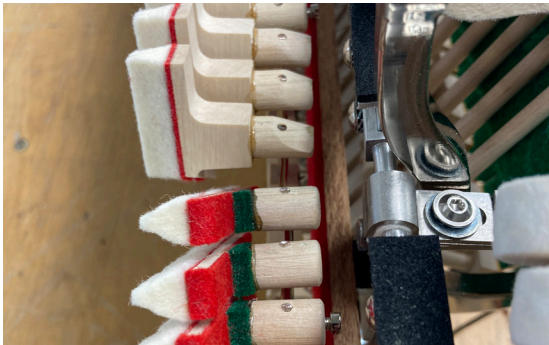
Replace the slotted screws in the damper drums with the set screws.
