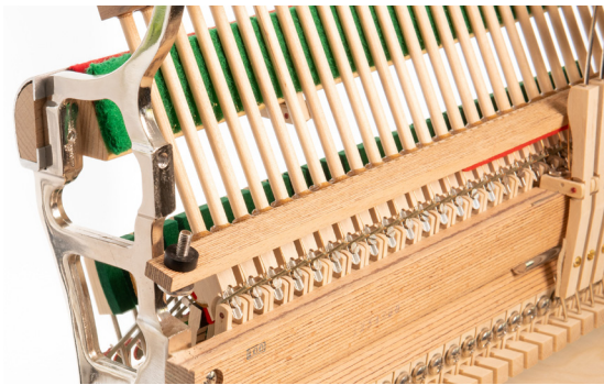
Removing the damper slap rail.
