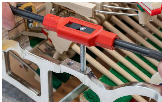
Cutting an M5 thread.
