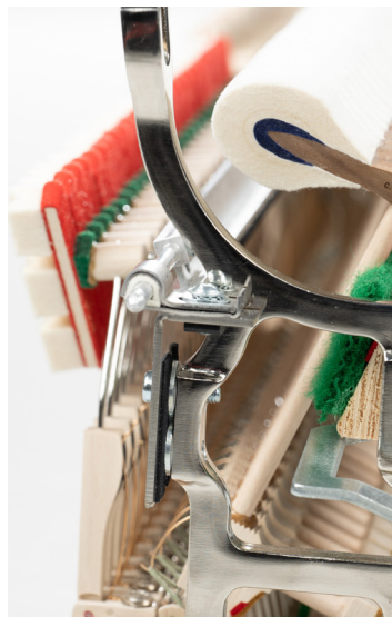
Washers between fixing bracket and action bracket.
