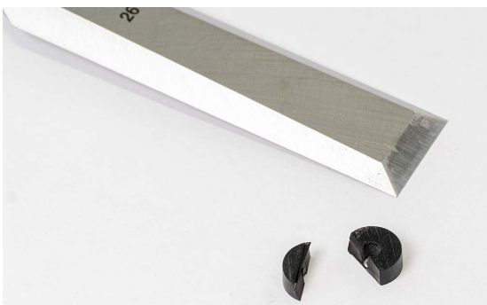
Cutting the rubber spacers.
