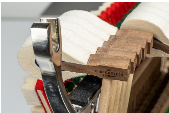
Distance of the hammers to the stop rail.
