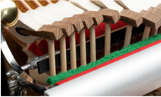
Stop rail in a right angle to the hammer shank.
