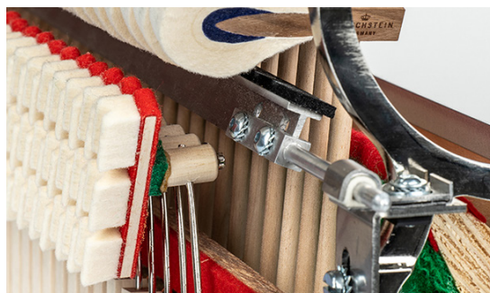
Distance between stop rail and damper drums.
