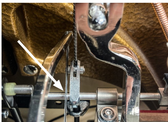
Shorten the stop rail shaft, deburr it and remove the metal chips.
