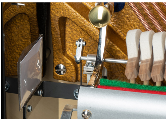
Stop rail switched on.
