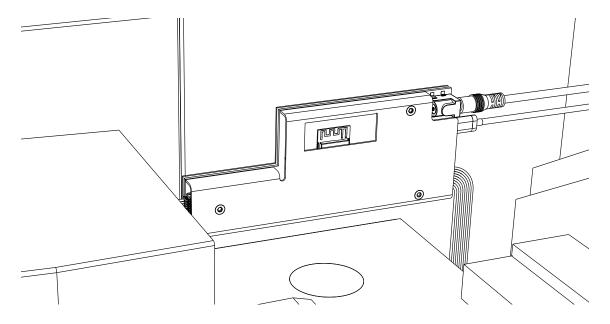
Use the self-adhesive cable clamps (CBD-00024) to fix the cables to the to the key bed.
