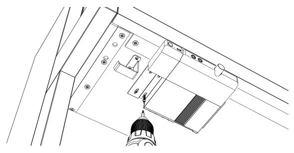
Attach the VARIO duet module (VE03001000001/ VE03001000002) directly to the right of the VARIO connect+ module with four screws (VE00002000001/ CBD-00055).
