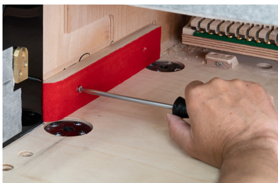
Unscrew the bumper strip.
